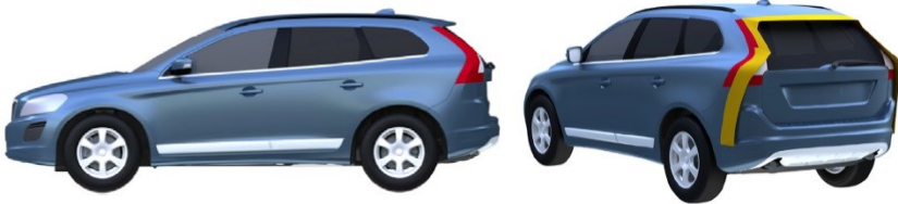
Fig. 3. Rear view of the smooth extensions, configuration B.
