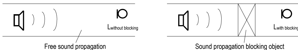
Arrangement to determine the insertion loss of an object
