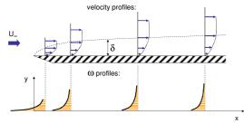
Vorticity is continuously produced on the wall surface due to the no-slip condition, and it is conducted into the main stream by the viscosity.
