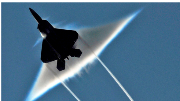
Wave patten around an F22 aircraft
