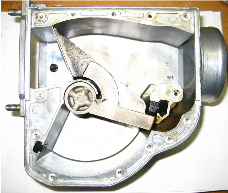
Figure 1.5 – The AFM – flap is closed
