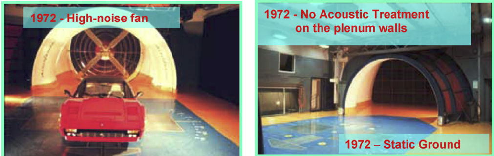
Fig. 1. A view of the original wind tunnel, as built in 1972. Typical features, the high-noise fan, the static ground and the absence of acoustic treatment on the plenum walls.
