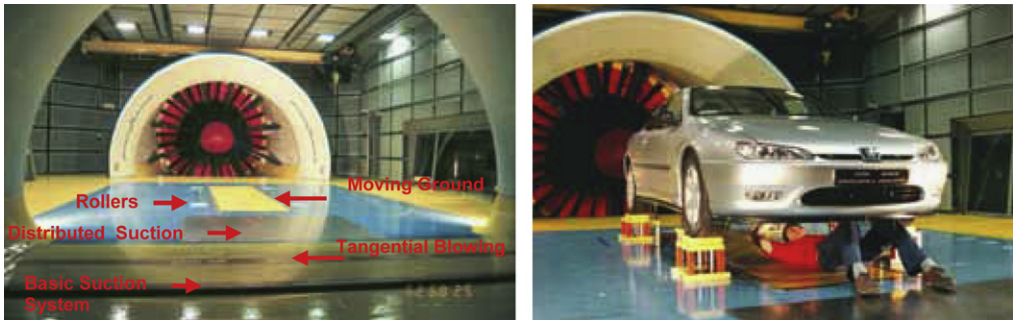
Fig. 5. The ground effect simulation system. The moving ground, the rollers, the suction and blowing subsystems, the car supports and the car lifters.
