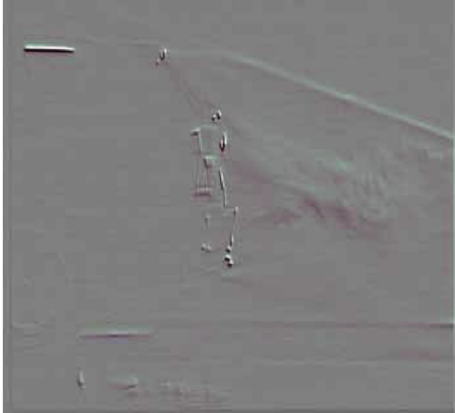
Fig. 25. Backlight soiling. Visualization by laser light-sheet and smoke on laser light-sheet and smoke on the car centerline.
