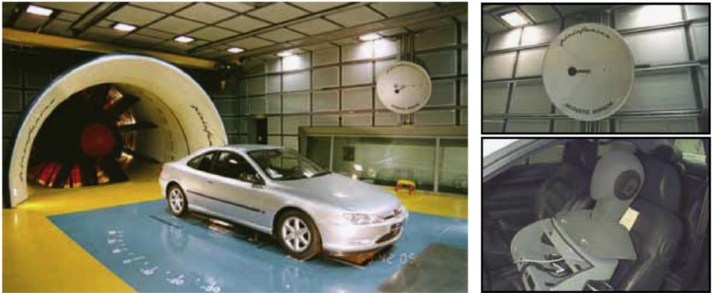
Fig. 3. (a) Acoustic heads to measure the noise inside the car and ellipsoid acoustic mirror and its traversing system on the test section wall.
