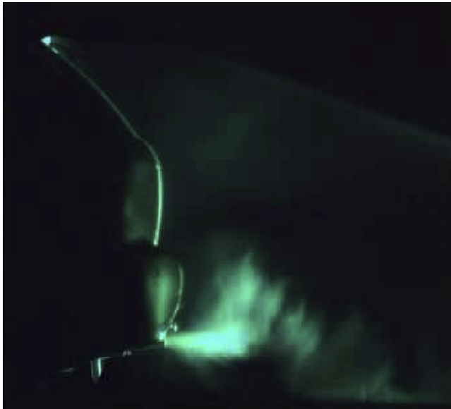
Fig. 24. Recirculation of exhaust gases.
