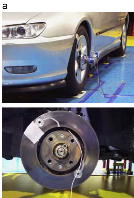
Fig. 27. (a) Sensors on the brake disk for cooling measurement.
