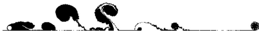
Fig. 20. Final position of the vortices for the flow past a circular cylinder in moving ground for h/d=0.05 at Reynolds number of 1.0 \times 10^5 .
