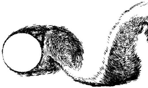
Fig. 12. Near wake behaviour using moving ground at an instant represented by point B for h/d=0.45 .
