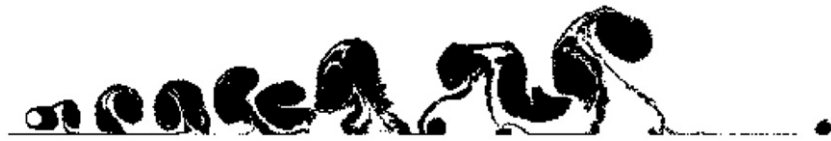
Fig. 19. Final position of the vortices for the flow past a circular cylinder in moving ground for h/d=0.45 at Reynolds number of 1.0 \times 10^5 .
