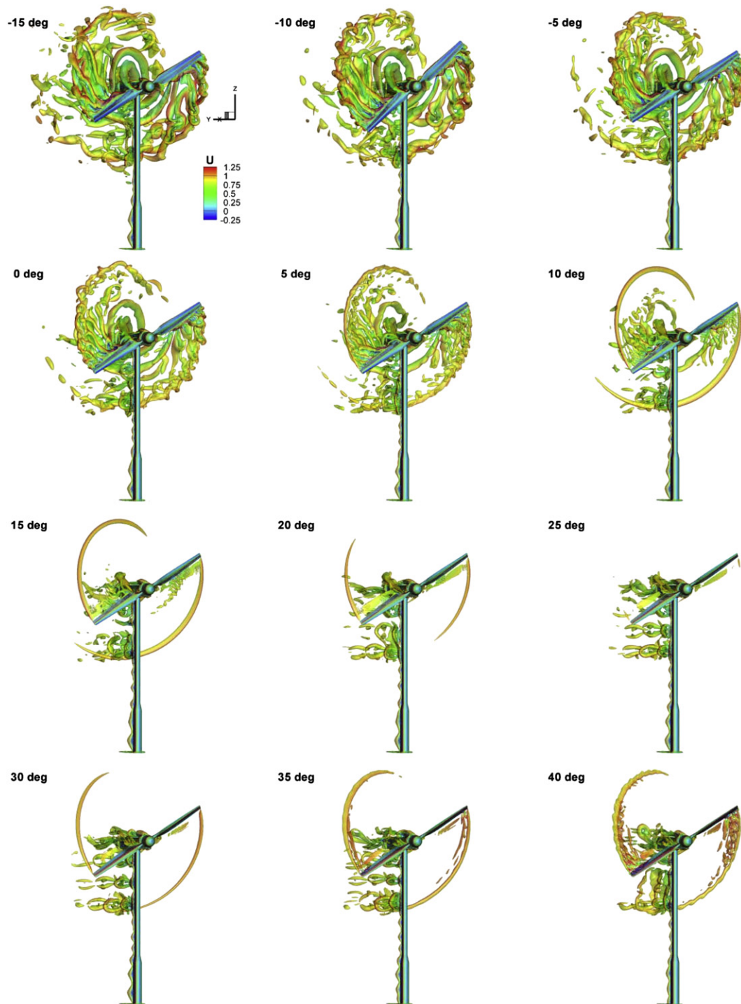
Fig. 11. Vortical structures represented by iso-surfaces of Q = 5 for different pitch angles (wind velocity 15 m/s).
