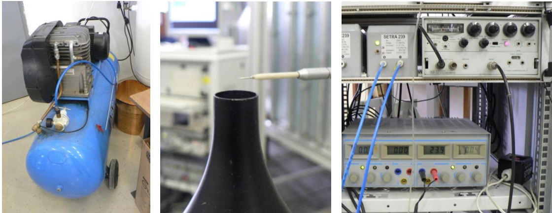
Figure 19 - Hot wire calibration
