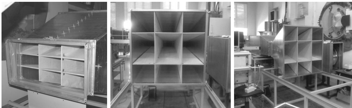
Figure 41 - Split-level diffuser construction
