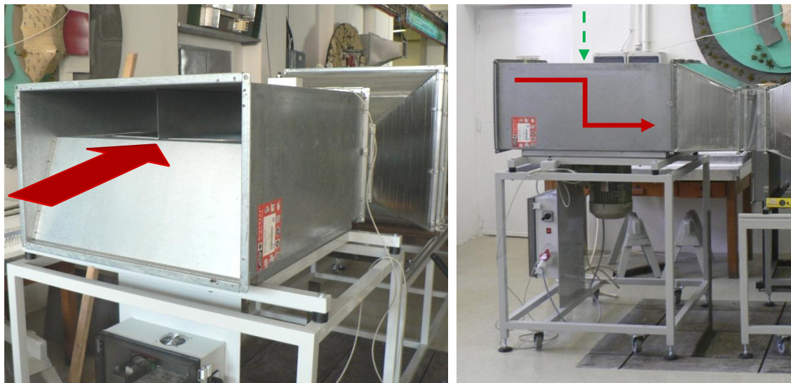
Figure 23 - Original suction design (red arrows) and optimal case (green arrow)
