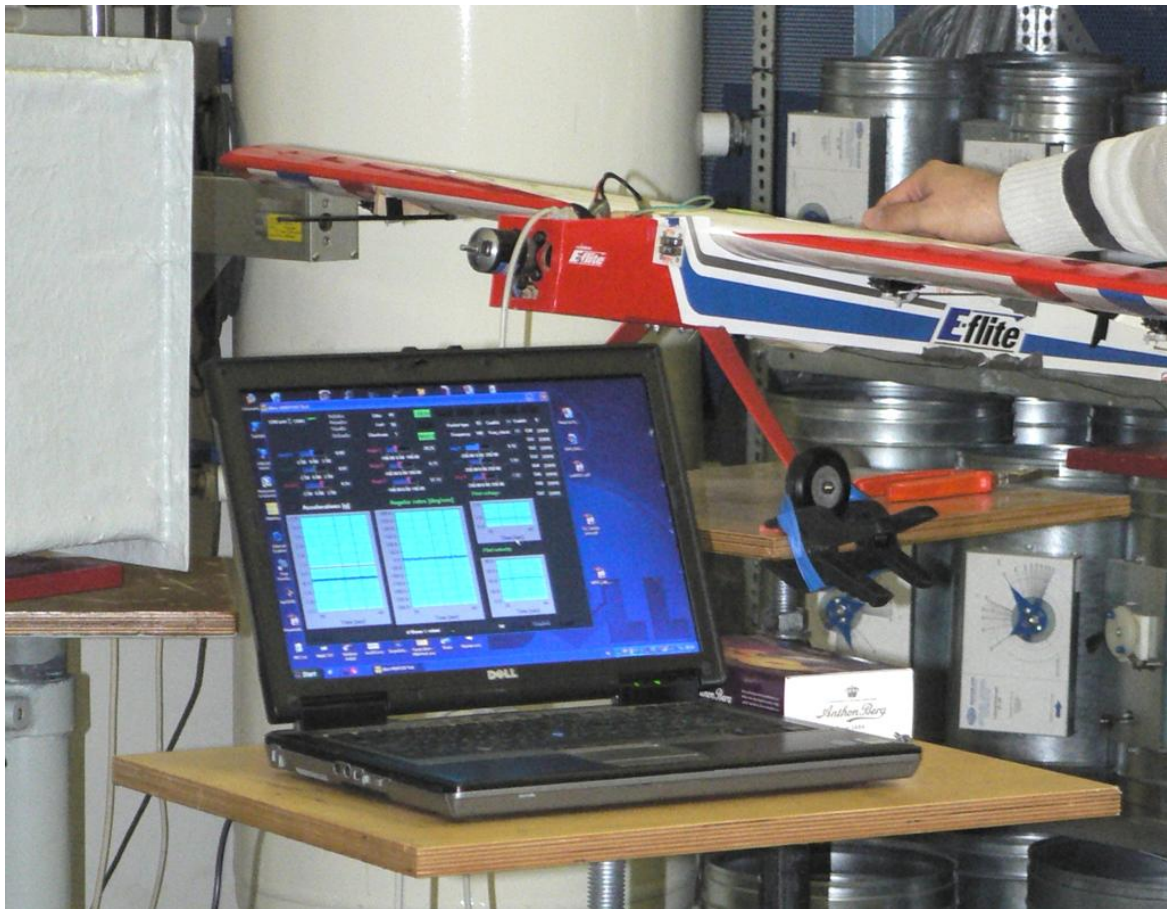
Figure 57 - RC airplane velocity sensor calibration
