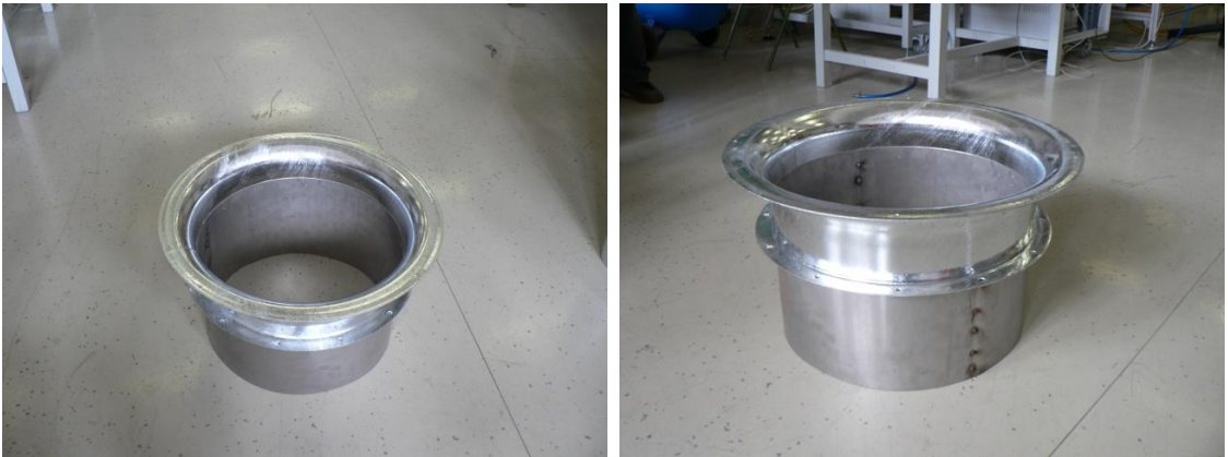
Figure 27 - Suction cone with additional tube section
