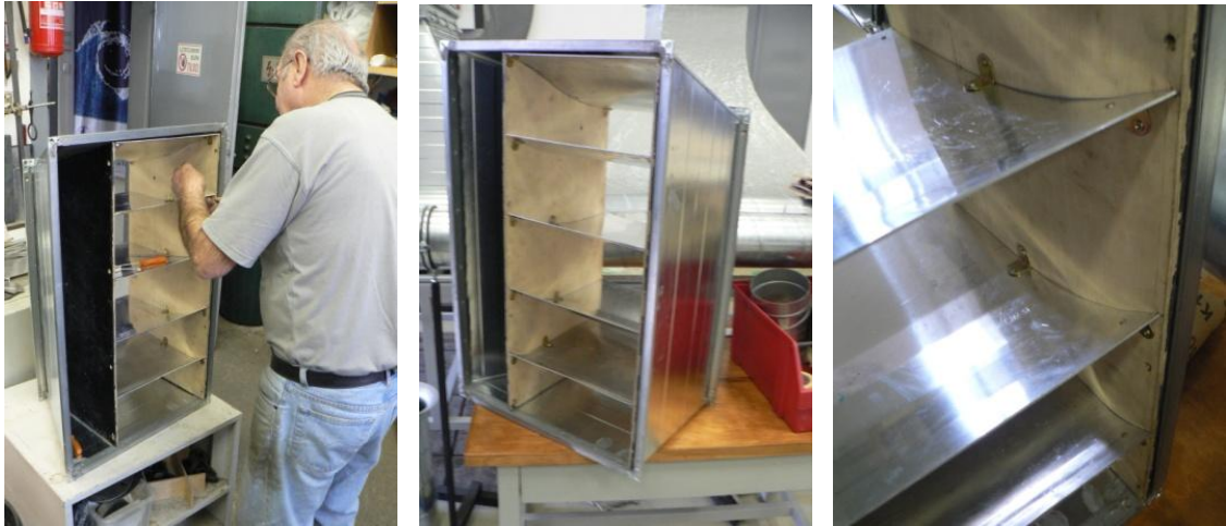
Figure 10 - Manufacture of vane series
