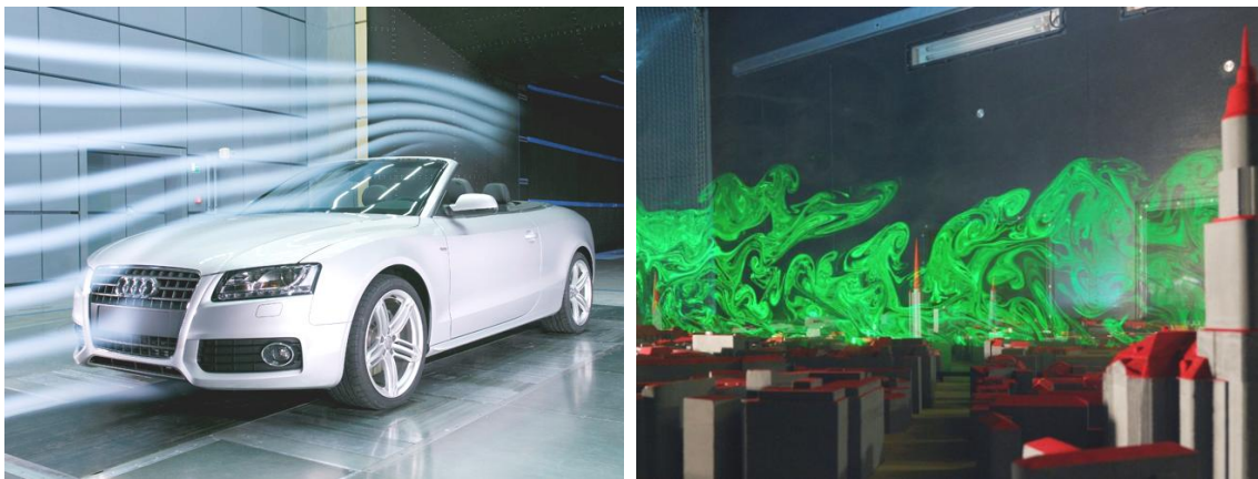
Figure 1 - Flow visualization around a real vehicle [1] and around a city model [2]
