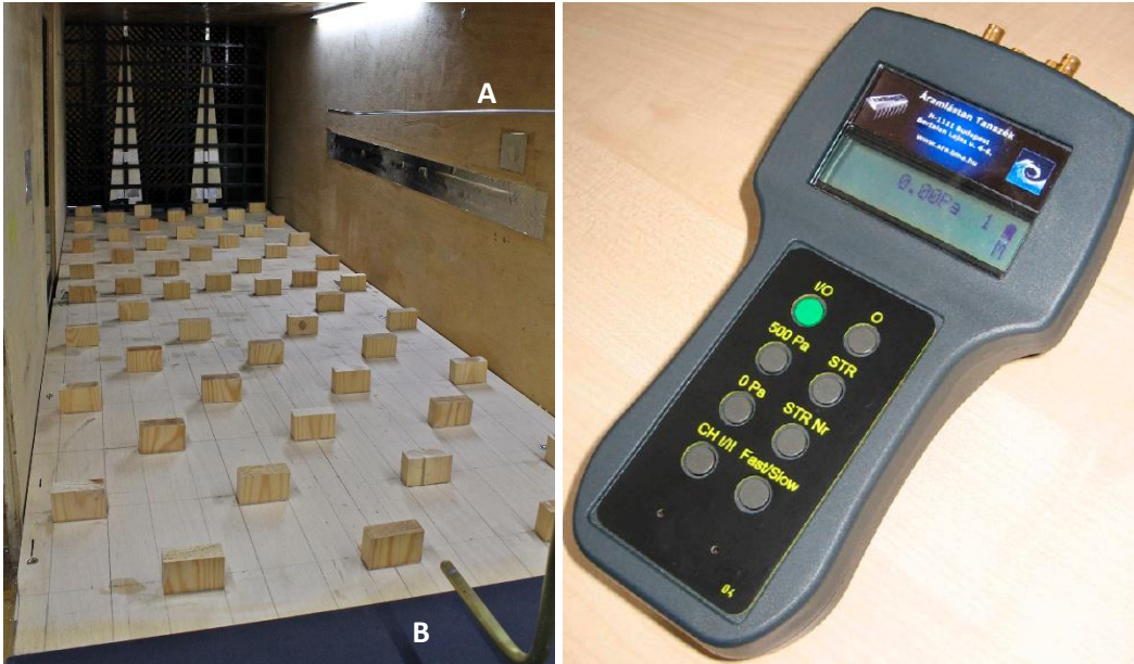
Left: Boundary layer generation. A: reference Pitot-static tube (at z = 300 mm height) B: vertically traversed Pitot-static tube for velocity profile measurement. Right: EMB-001 Handheld device to measure differential pressures.
