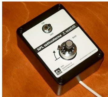
Wind tunnel speed controller
