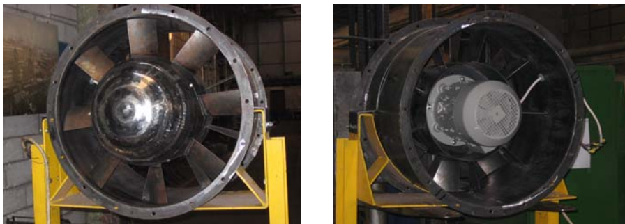
Fig. 2.2. The above fan with hemispherical nose cone. Front and rear views (direct drive, outlet guide vanes)
