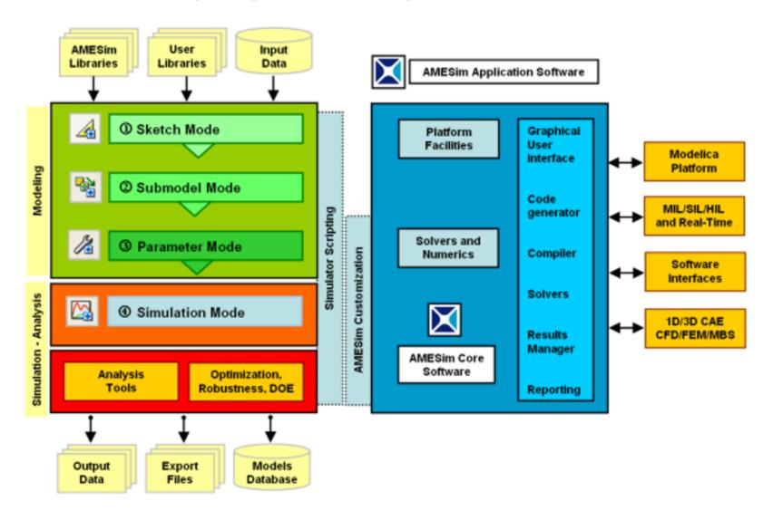
AMESim is a 1D lumped parameter time domain simulation platform.
