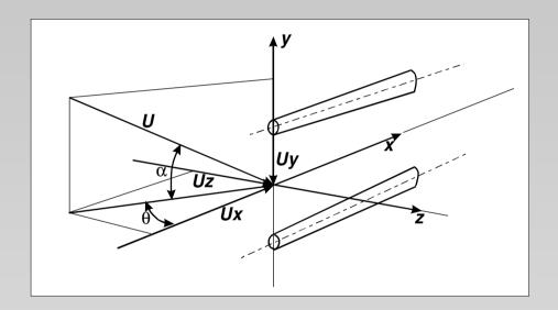
Velocity vector *U* is decomposed into normal *Ux*, tangential *Uy* and binormal *Uz* components.
