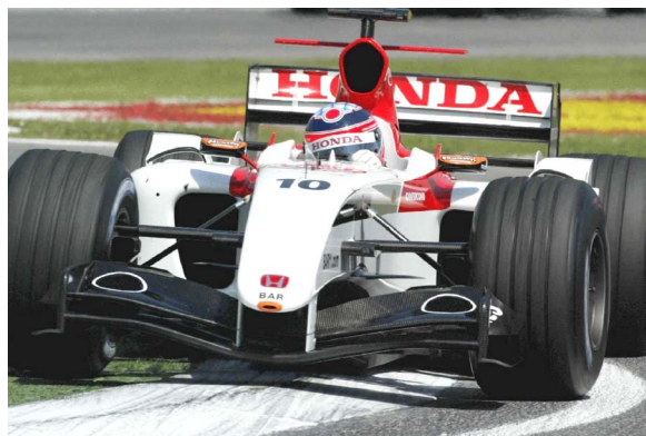
Fig. 2 An illustration of a race car front wing equipped with end-plates and Gurney flaps, and race car wheels
