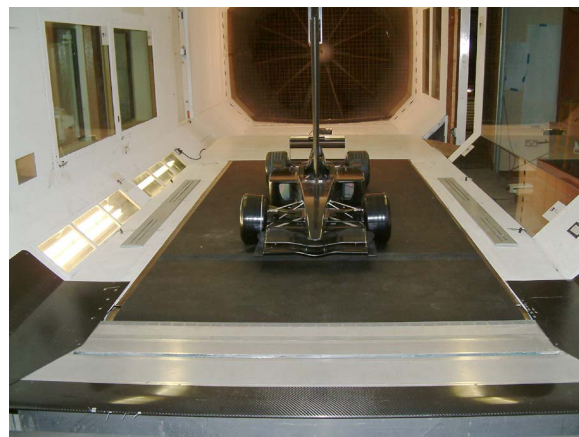
Fig. 6 Image of a race car model in a low speed wind tunnel equipped with a moving belt system
