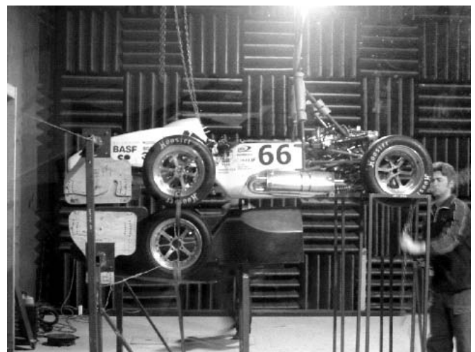
Figure 14: Full scale 'symmetry plane' test rig. Top: Front view, Bottom: Side view.
