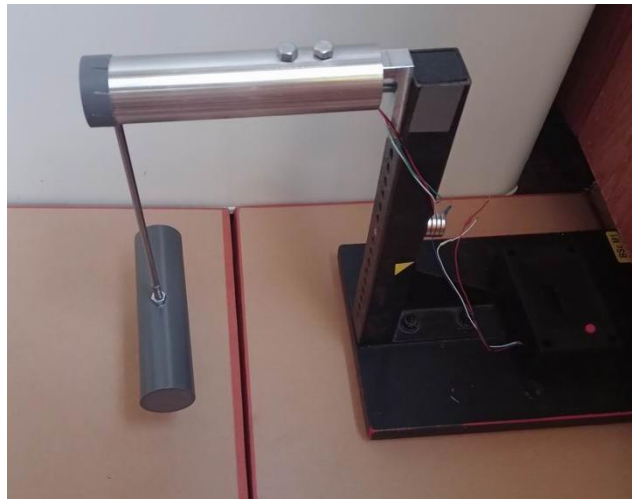
2 . Fig. Force measuring stand with the measuring stem hanging from it and a cylinder on it. The shiny tube is the windshield, inside it is the load cell/force gauge.
