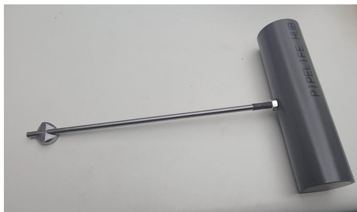
3 . Fig. Cylindrical body on the measuring stem. The steel component glued to the left end of the stem ensures a stable connection to the magnet, but also the ability to tilt it.
