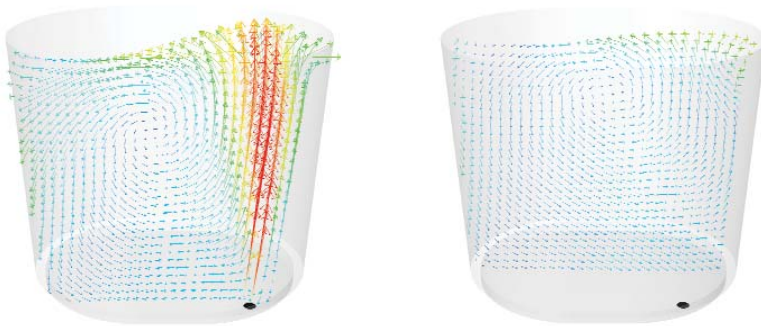
Velocity vector field on the argon plume (left) and center (right) planes of the ladle show that circulation is ongoing, even at a distance from the jet entrance
